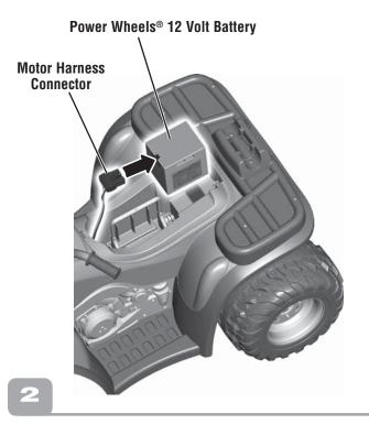
· Plug the motor harness connector into the battery.
